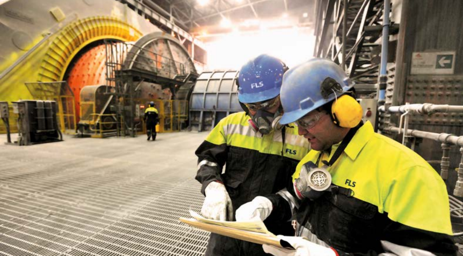
SAG mills provide the modern mining industry with workhorses able to manage most high throughput grinding tasks. Photo: FLSmith
