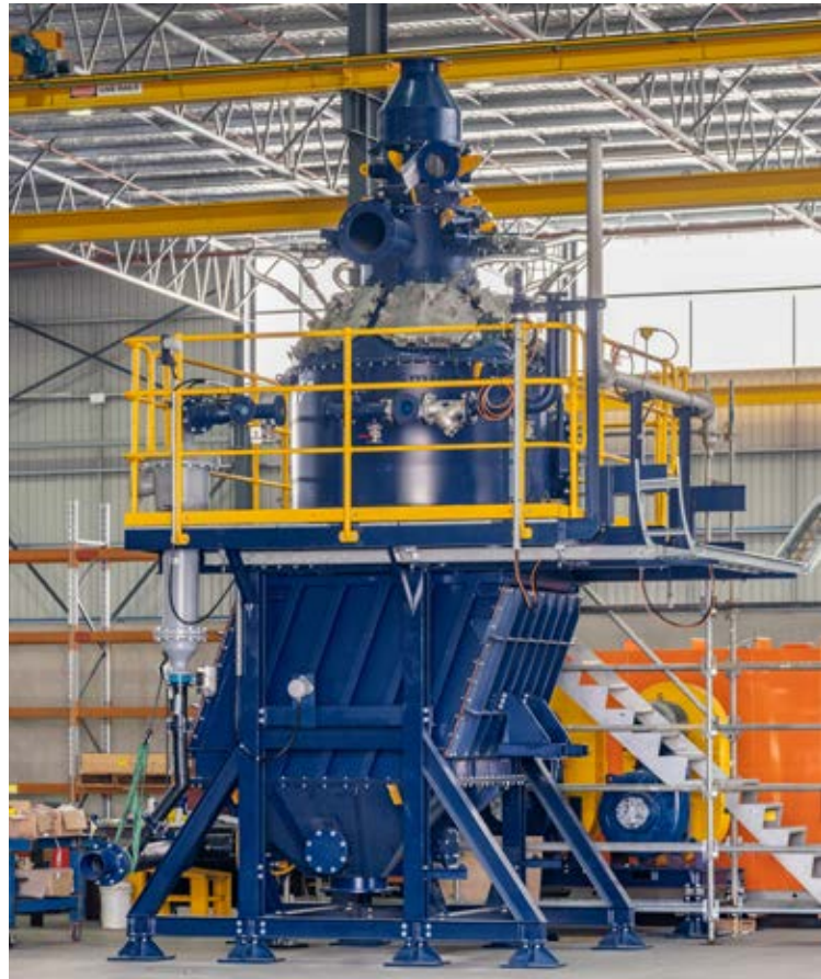
Coarse particle flotation technologies offer the opportunity to coarsen SAG circuit grind target and/or increase mill throughput. Pictured: FLS REFLUX Flotation Cell
