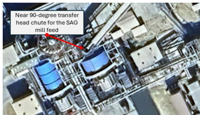
Figure 7 – Phu Kham’s near 90-degree transfer head chute for the SAG mill feed
