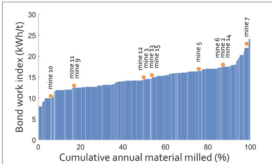
Figure 1 – Newmont sites on the Bond intensity energy curve, comparing the BWi
