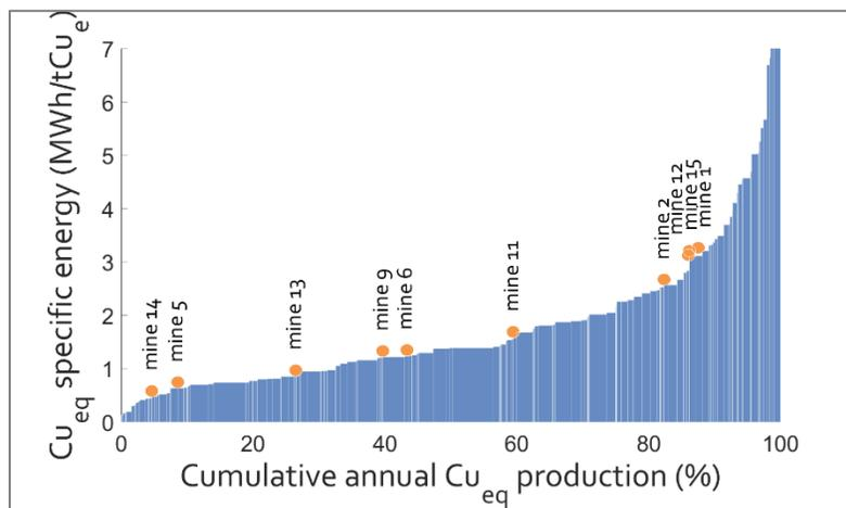
Figure 4 – Newmont sites on the grade intensity energy curve
