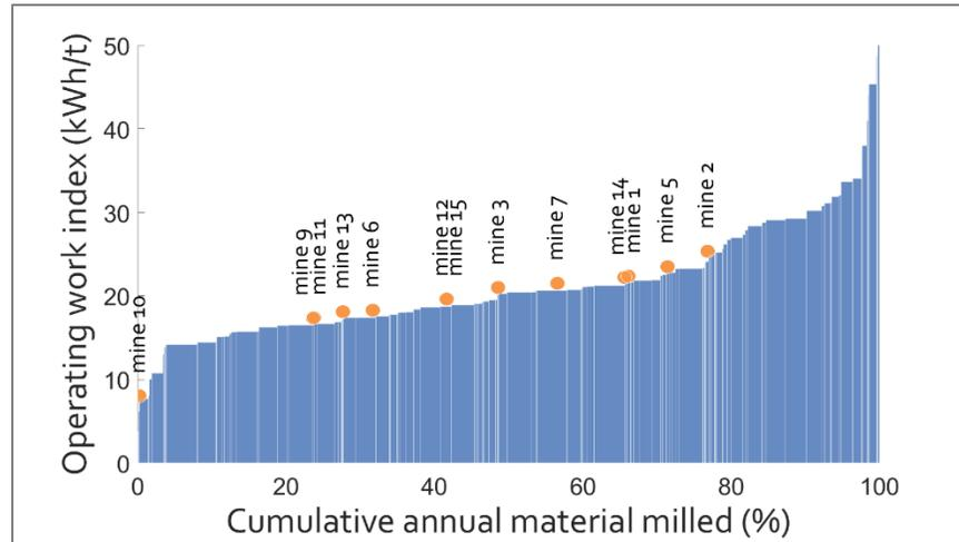
Figure 2 – Newmont sites on the Bond intensity energy curve, comparing the OWi
